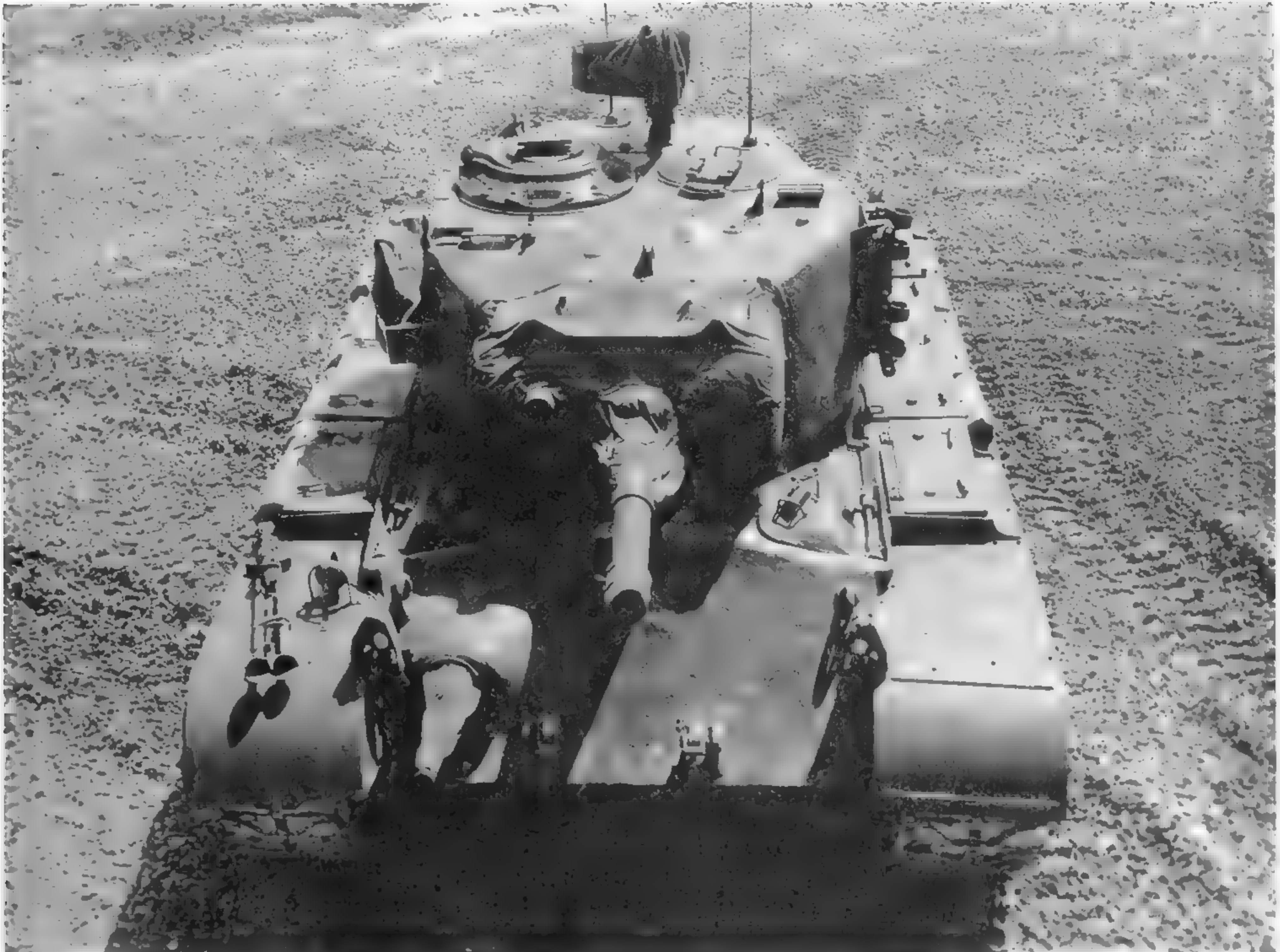
Here is the 105mm howitzer-armed M45. The bow and hull machine guns are both in their canvas covers, and the tripod for ground use of the commander's .50-caliber gun is stowed on the right front fender. (Photo courtesy of the Patton Museum)
